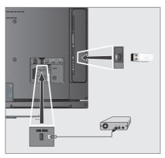
Connect the »USB HDD« socket of the television and the corresponding socket of the data medium (external hard disk) using a USB cable;
